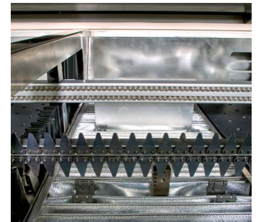
Chain conveyor: Enclosed width adjust module guarantees operation also under full load production conditions.
