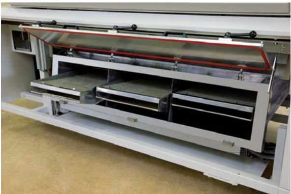
Innovative modular cooling concept for efficient and gentle PCB cooling.
