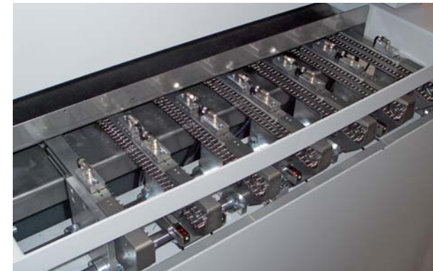
Uni-directional conveyor – 6-lane
