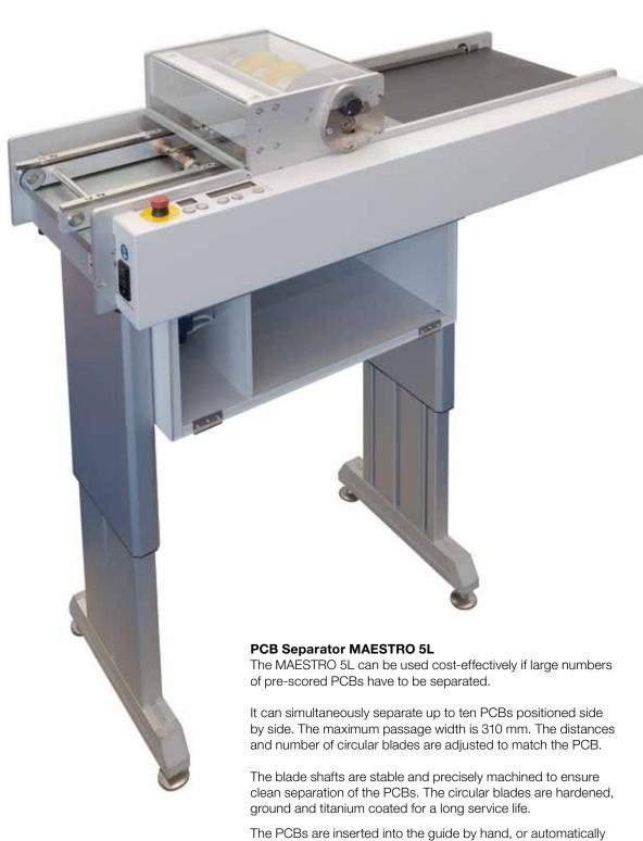
The PCBs are inserted into the guide by hand, or automatically by a loading station or an external conveyer belt. After separation, the PCBs are placed on the installed conveyor belt. The machine can be installed in an assembly line in conjunction with a SMEMA interface.
